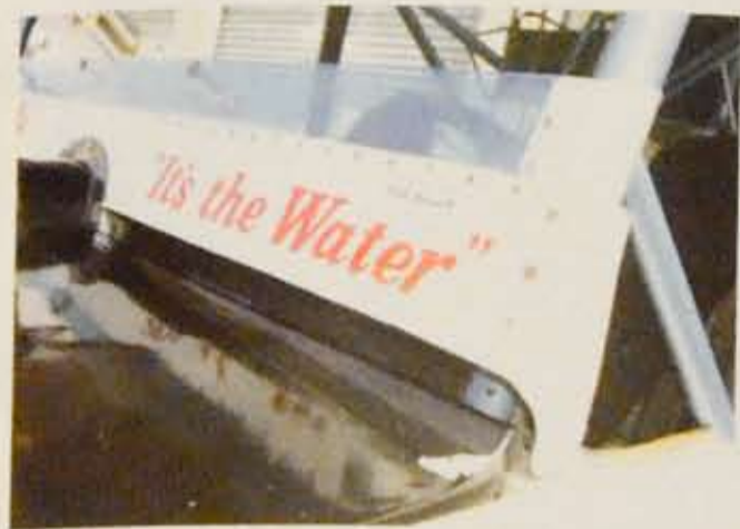
▲ A lot of innovative thinking went into the original Big Oly. At the lower end of the front window opening, an intake channel scooped air and directed it upward through a dual-pane Plexiglas shorty windshield. This created an air curtain that kept a lot of dust out of the cab.
