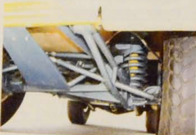
▲ The front suspension is a custom variation of Ford's Twin I-Beam. Instead of coming from the rear, the radius arms pivot from the front for better bump compliance. The steering linkage is also completely custom: the steering box is mounted aft of the coil spring and operates one end of a bellcrank, which in turn pivots the tie rods left and right.
