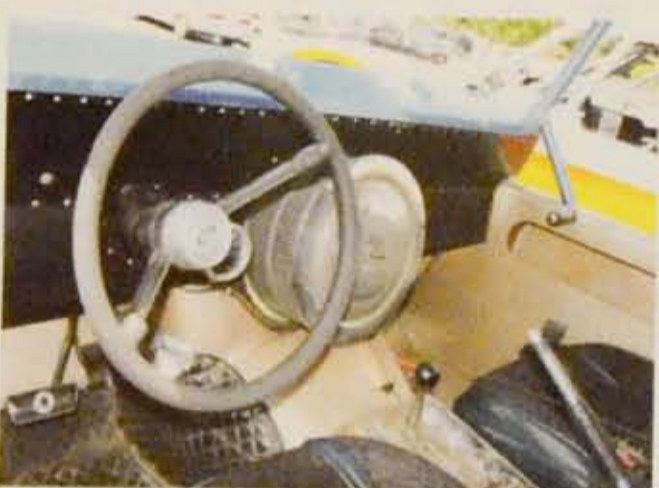
▲ Putting the air intake in the cab is a time-honored way to keep the filter from clogging when things get dusty. What looks like an E-brake lever is actually an adjuster for the trailing edge of the overhead wing. Adjusting the trailing edge up or down increased the aerodynamic downforce on the vehicle. Considering the Bronco's short wheelbase, vehicle control at high speeds was no laughing matter.
