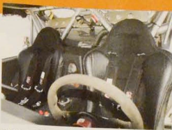
▲ Driver and co-driver have plenty of legroom and sit securely in PRP seats with matching PRP harnesses. A MOMO steering wheel, Auto Meter gauges, and a Lowrance GPS unit are popular items because they're durable and race-proven.
