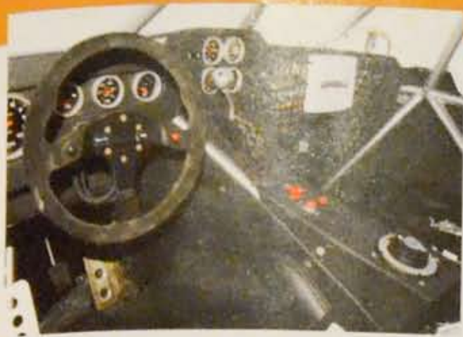
▲ Driver and co-driver have plenty of legroom and sit securely in PRP seats with matching PRP harnesses. A MOMO steering wheel, Auto Meter gauges, and a Lowrance GPS unit are popular items because they're durable and race-proven.
